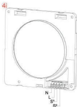
Take the internal wall-mounting part (4i) and the tools necessary to connect the main supply to the terminal box. Connect properly and safely the Live wires to the terminal block identified as “N” and “L”.
