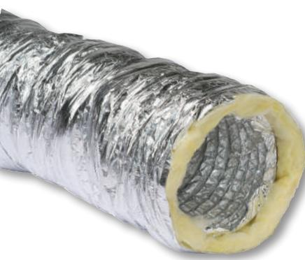
With an inner ply of micro-perforated aluminium/polyester, an insulating glass fiber and/or polyester fiber mattress (thickness: 25 mm, density: 16 kg/m<sup>3</sup>) and an outer aluminium/polyester protective layer. Suitable for many ventilation, air-conditioning and heating applications.
